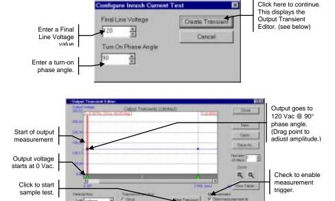
You can use the transient editor to make any final adjustments to the inrush current measurment such as fine tuning the width of the transient step, or positioning and enabling the measurement trigger.
