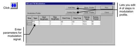
Modulation signals are comprised of from one to 20 individually programmed steps that may be combined into a modulation sequence and then run. Each step programs the modulation signal for the duration of the step. The amplitude and frequency of the modulation signal may be constant, swept linearly, or swept logarithmically from the starting value to a stop value. The sweep period is programmed in seconds.
