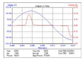
To save the waveform that appears in the display, select **Save Waveform** in the File menu. This saves the displayed waveform as an ASCII file, which can be easily imported into other application programs.
