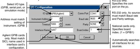
If there seems to be no communication between the Agilent AC Source GUI and the ac source, select **Auto Detect** to detect any ac sources connected to your pc. Also try resetting the I/O interface by clicking the red reset button. This also resets the ac source to its default settings.
