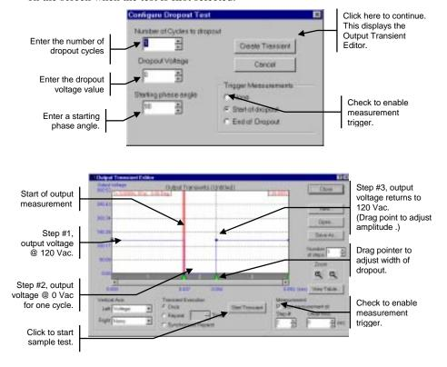
You can use the transient editor to make any final adjustments to the ac line dropout test such as fine tuning the width of the dropout, or positioning and enabling the measurement trigger.
