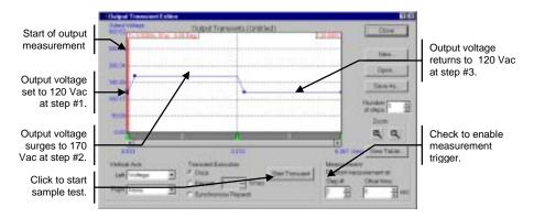
You can use the transient editor to make any final adjustments to the ac line surge/sag test such as fine tuning the slew rates of the surge or sag, or positioning and enabling the measurement trigger.
