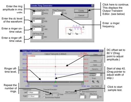
You can use the transient editor to make any final adjustments to the telephone ringer waveform such as fine tuning the dc level of the waveform. Note that the transient editor only displays the rms-portion of the telephone ringer; it does not display the actual waveform.
